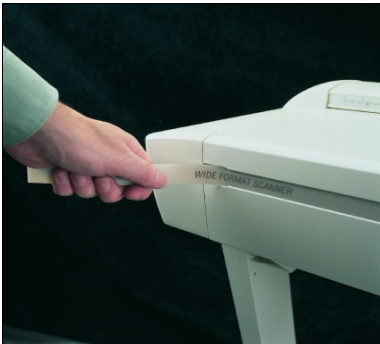
Figure 3-4 Access the DIL-switches
